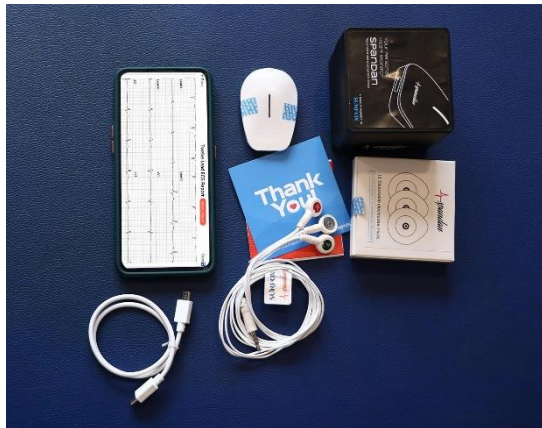
Fig. 1. Spandan portable ECG developed by Sunfox Technologies Pvt. Ltd.
